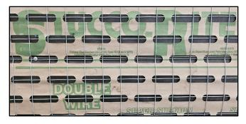
Stucco Rite products install in one step, replacing the traditional three-step process of line wire, asphalt paper and rolled wire lath.
