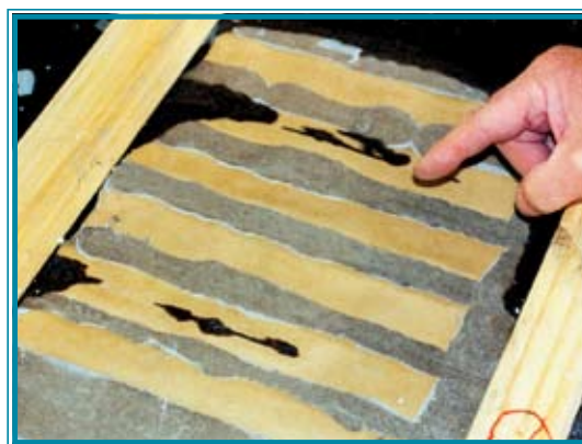
Fig. 2 Wire Mesh showing Internal Coverage and embedment of wire
